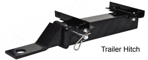
Using 8x25mm hardware provided, attach brackets to hitch using the inside holes. Bracket should face each other as shown.
