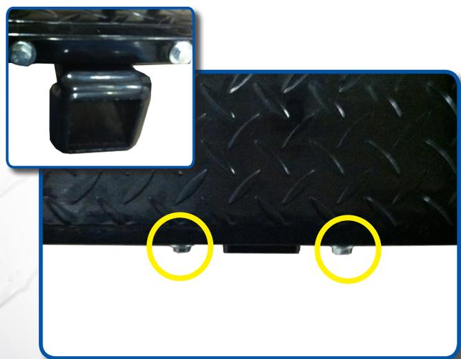
Using 8x40mm hardware, attach trailer hitch to footrest as shown.
