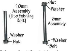
5. Secure Brush Guard with washers and nuts as shown. Tighten Nuts.
