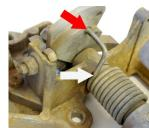
Remove and retain the nut from the brake pedal shaft. Do <u>not</u> remove the shaft.
