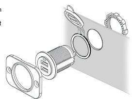
5. Use (2) spade connectors (not included) to connect your wires to the back of the outlet. Connect the positive (+) wire to the positive (+) terminal and the negative (-) wire to the negative (-) terminal. Terminals are marked positive (+) and negative (-).
