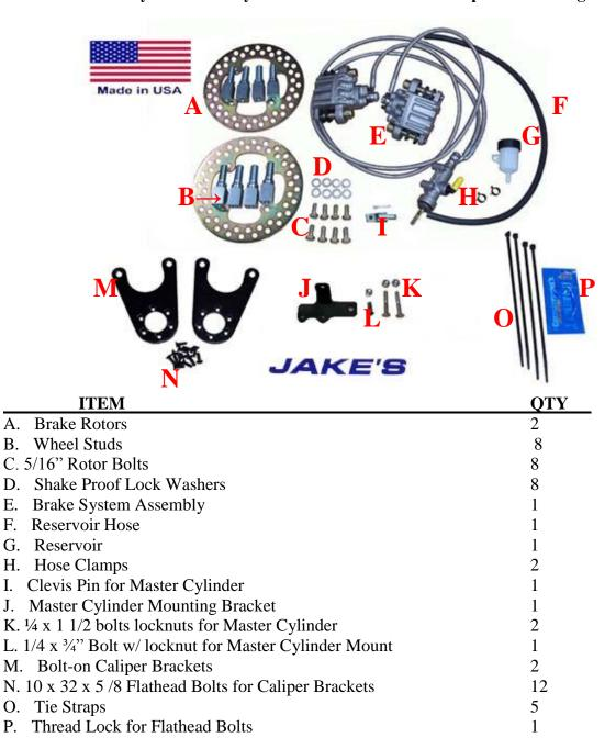
NOTE: This is a sophisticated system. We pre-charged the lines to save massive brake bleeding. We recommend this kit be put on by mechanically trained professionals or someone with hydraulic brake experience! System may need bled if you allow air to get in the reservoir line when installing.
