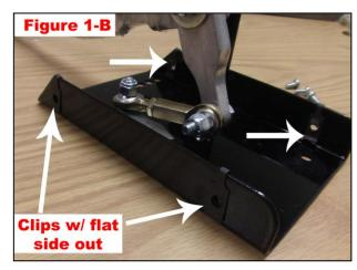
tabs on the outer shifter cover as shown in FIGURE 1. With the flat side of the clips to the outside, snap
