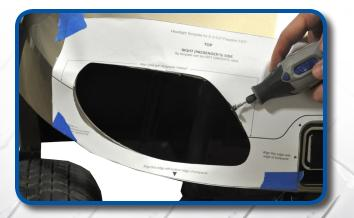
Cut out the shape of the headlight.Use the cutting tool to remove the excess trim. \*Flip template over repeat process on the other side. Use sandpaper to smooth out any rough edges. Mount headlight through the cutout. Push top half in first as shown.
