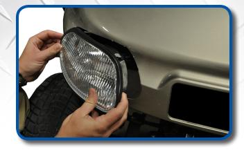
\*Make sure cart is in TOW mode. Lift front of the cart and place jack stands to support. Feed front harness down through
