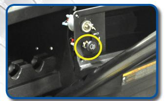
Attach the nut to tighten the switch. Reattach Push/Pull knob. Using retained hardware from Step 12, reattach dashboard.
