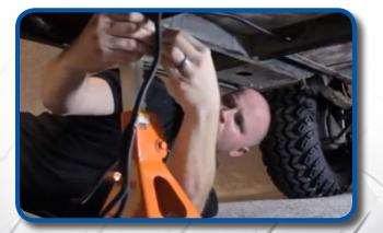
Remove the Push/Pull switch from harness. Run the wire harness through the holes under the frame to secure the harness.\*Use the zip ties provided. Attach headlight to wire harness as shown. Secure excess wire with zip ties.
