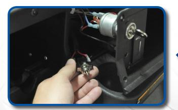
Feed the Push/Pull switch wire through the dashboard.
