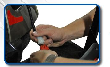
Feed the tail light harness through the back of the cart. Attach rear tail light wire harness as shown. Secure wire with ties.
