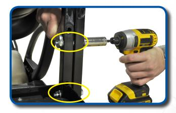
Install Expandable cargo box using retained hardware from step 1 and tighten.
