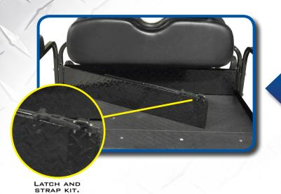
To secure cargo box, fold Passenger side panels in first, then drivers side.
